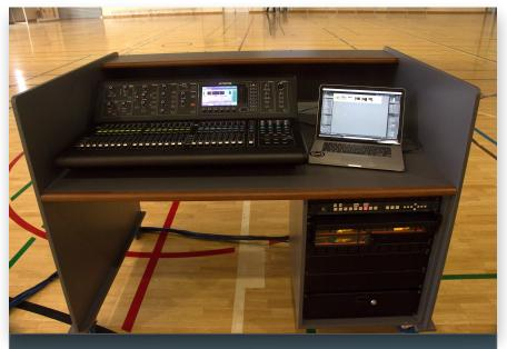
Custom mobile equipment operation console, included: Midas M32, wireless microphones and vision presentation switcher
